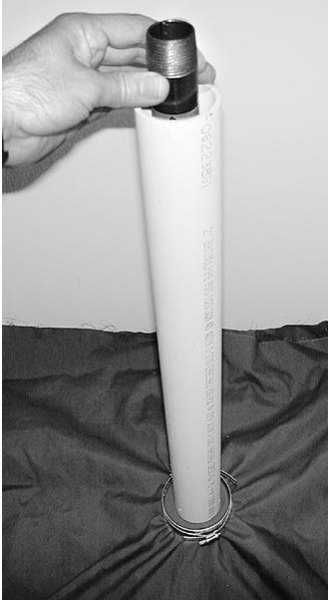
Figure 3. Drop Tester just before making a test drop. Note that the guide tube is centered on the clamped fabric, and the drop probe is being used as a plumb bob to make the guide tube vertical.
