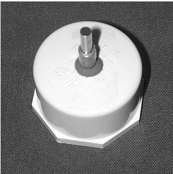
Figure 2. Plastic cap with gage pin and drill collar sticking out, all epoxied together (gray).
